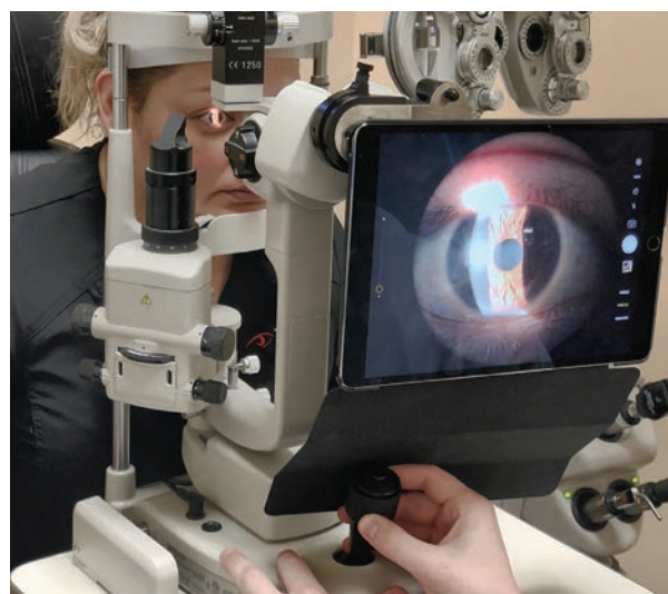
Figure 6. An attached tablet for taking photos. Specific adapters are manufactured for different types of slit lamps.
